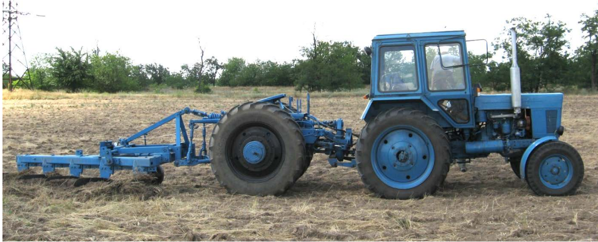
Fig. 2. The tillage unit on the basis of a modular power unit
