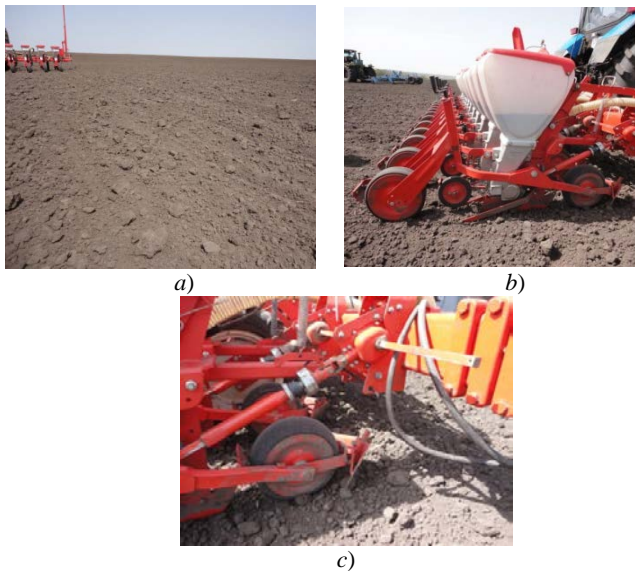
Fig. 1. Typical condition of field surface before sowing sugar beet: a – poor quality of the soil processing in terms of soil aligned and lumpiness; b, c – the work of sowing drills sections under unsatisfactory conditions
